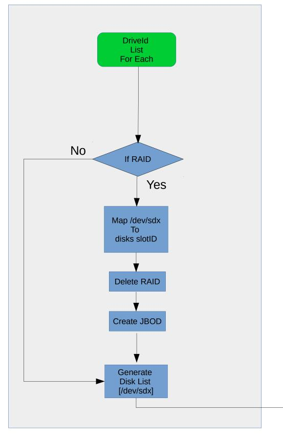
Erase Command Module (Each disk have such module running in parallel)
